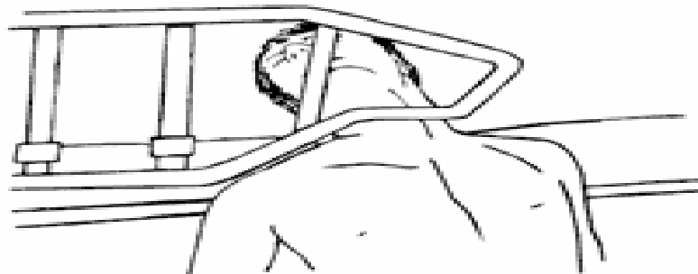
Zone 4 - Entrapment between top of compressed mattress and bottom of rail at end of rail
