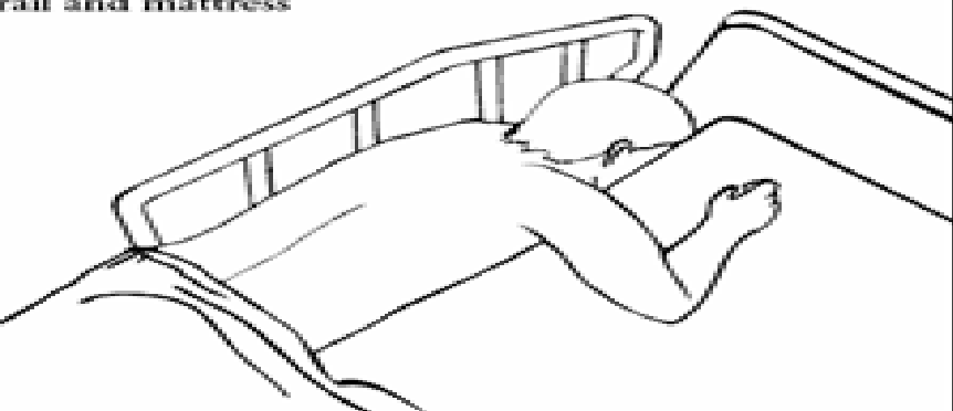
Zone 3 - Entrapment in horizontal space between rail and mattress
