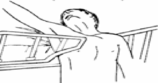
Zone 5 - Entrapment between split rails
