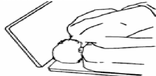
Zone 7 - Entrapment between head or foot board and mattress
